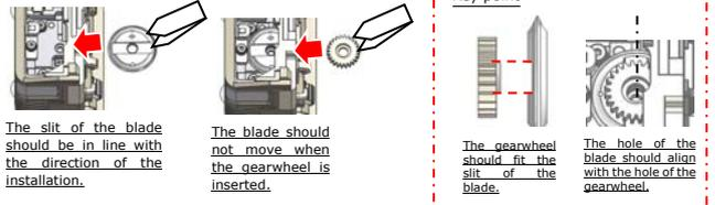
The slit of the blade should be in line with the direction of the installation.
