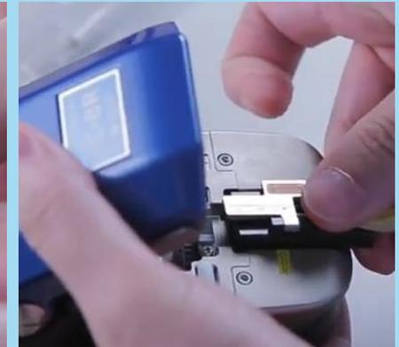
Remove the buffer and cleave the fiber.
